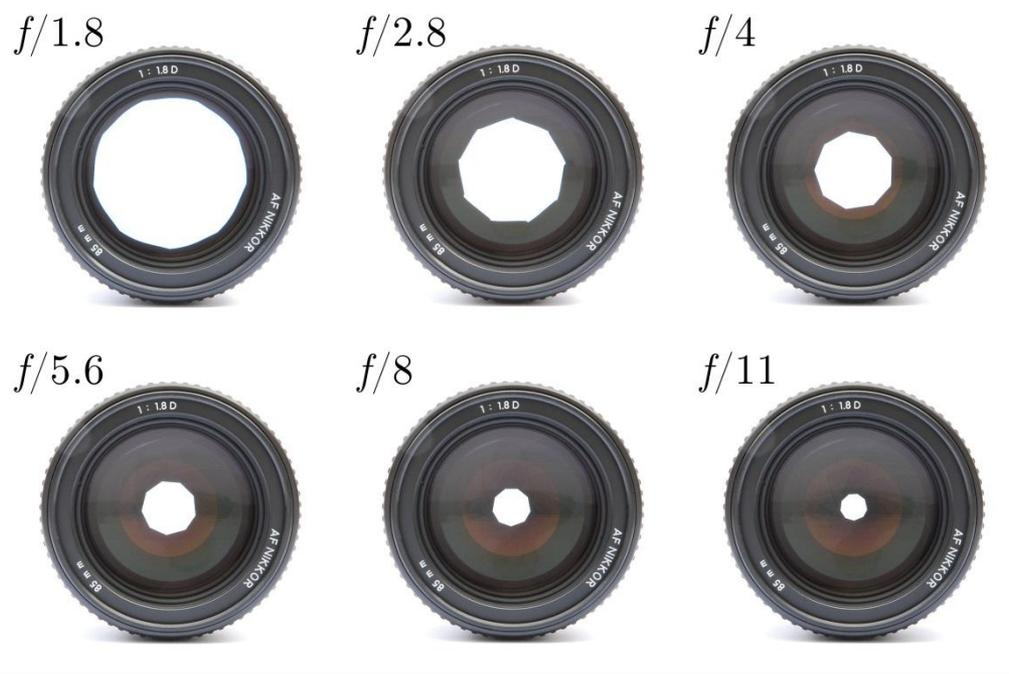
Here a open lens (left) closed lens (right)
